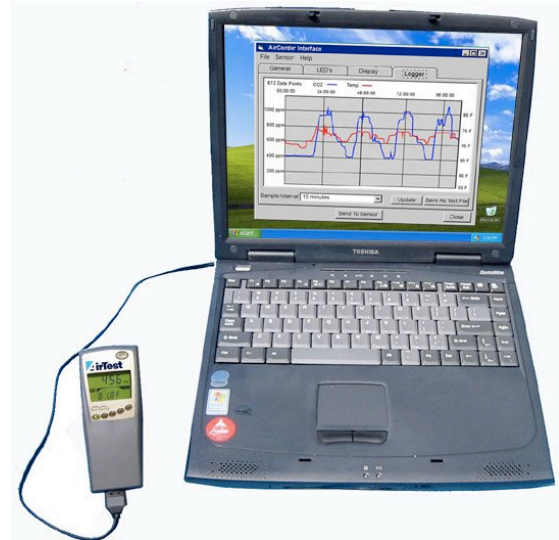
Now You Can Measure And Trend Log Fresh Air Ventilation In Every Zone
